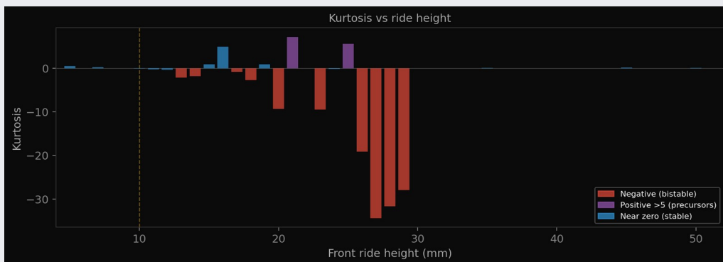
Figure 3. Kurtosis versus ride height. Negative values flag candidate bistable ride heights for closer inspection; positive values mark spike-like behaviour; near-zero is usually more stable. The plot's practical value is telling you which neighbouring CFD cases to compare in the 3D flow field.
